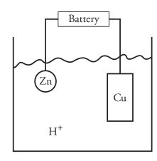
Pennies are made primarily of zinc, which is coated with a thin layer of copper through electroplating, using a setup like the one above. The solution in the beaker is a strong acid (which produces  $H^+$  ions), and the cell is wired so that the copper electrode is the anode and zinc penny is the cathode. Use the following reduction potentials to answer questions 29-31.
