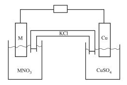
The cell potential is found to be +0.74 V. Separately, when a bar of metal M is placed in the copper sulfate solution, solid copper starts to form on the bar. When a bar of copper is placed in the MNO<sub>3</sub> solution, no visible reaction occurs.
